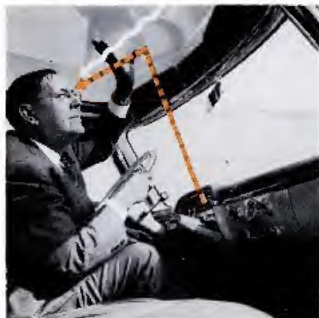
Plastic roof lets sun glare through (wavy line) and reflects instrument lights at night (dotted line)
